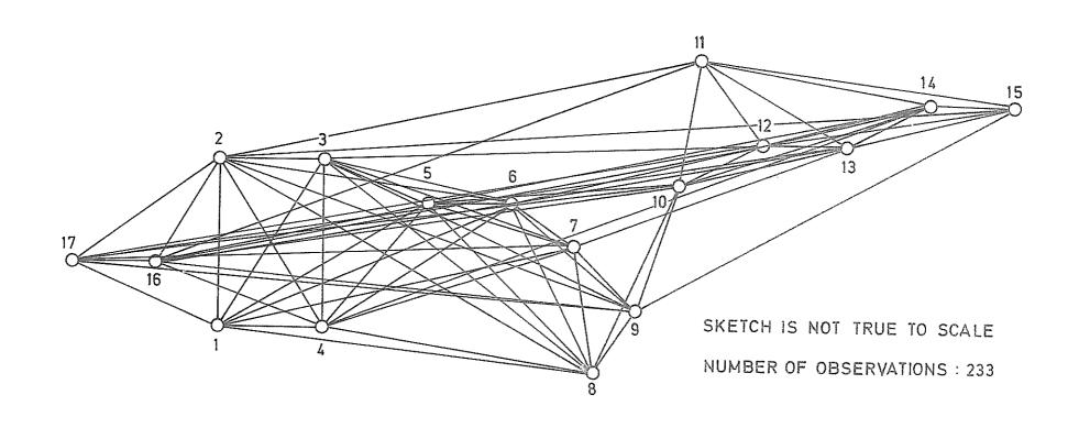
Fig. 1 : structure of gravity network Hannover 1976
