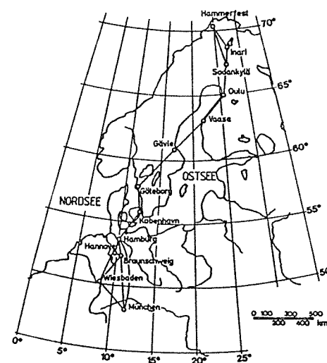
Fig. 2: Gravity measurements on the northern part of the European gravimetric absolute calibration line used for the gravity meter calibration system Hannover
