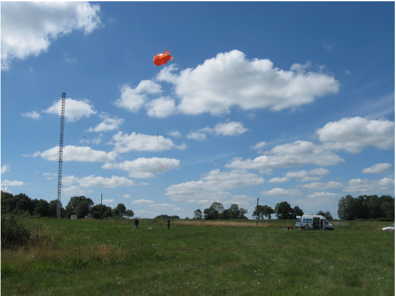
CNRM/4M is measuring turbulence with a tethered balloon close to the 65-m tower of Lannemezan. Monday 30 August 2010.
