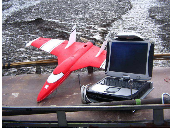
Figure 1: The Multiplex FunJet used as airframe for the SUMO system and the ground control station (laptop).
