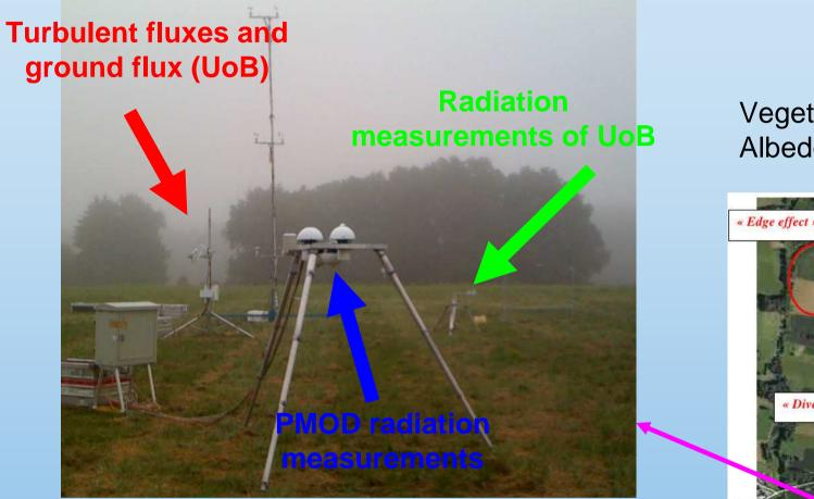
Measured parameters: Temperature,  $H_2O$ ,  $CO_2$ , radiation, wind, pressure, soil heat flux
