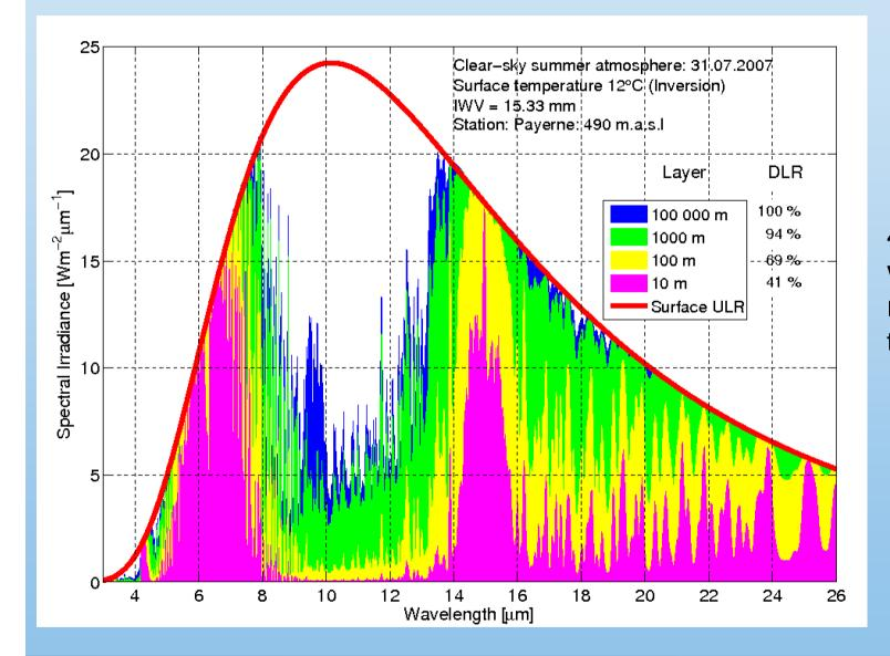
40 % of the downwelling long-wave radiation stems from the first 10 meters!
