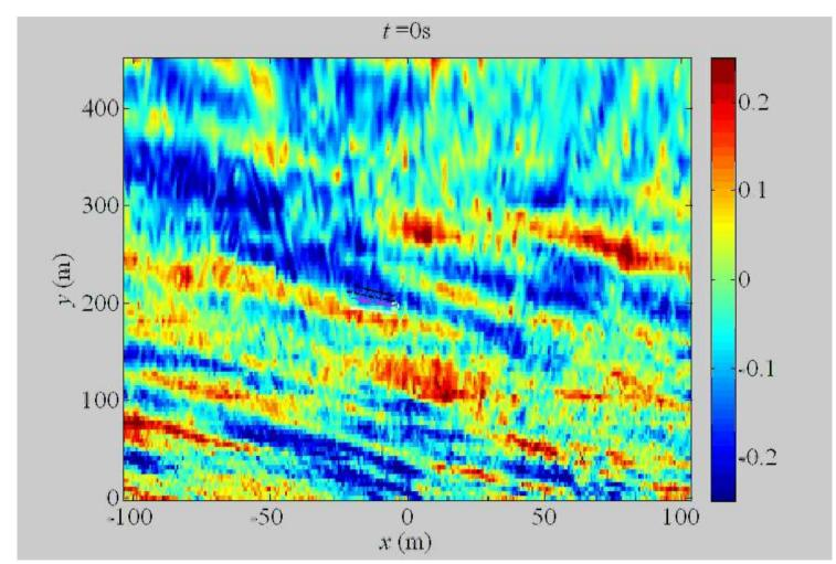
Turbulent structures in a convective boundary layer can be studied from high frequency **Fischile Co-berry** perature fluctuation. Here white circle is the position of the sonics.
