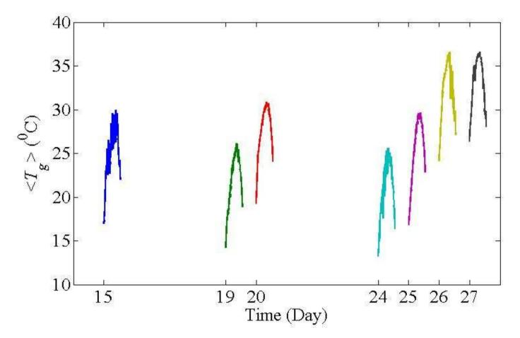
Plot of 5 min mean surface temperature (0600-1900 UTC) at divergence site. Surface temperatures are calculated assuming surface emissivity *Firenze*, 6-8/025
