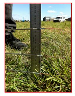
On IOP from 1800 LT to 1000 the next day. The height measurement was retaken for each deployment and was measured to the *hard-packed* soil surface. Hence, the lowest thermocouple was just at the top of the "grass canopy".
