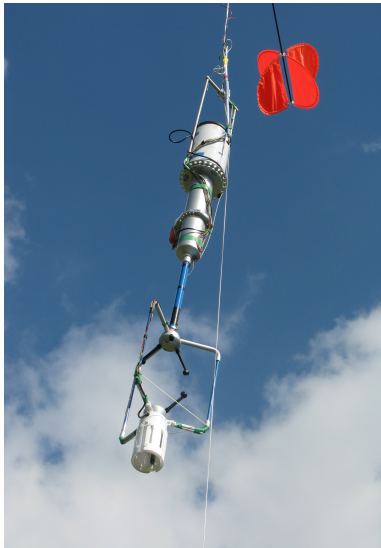
The turbulence tethersonde: sonic anemometer + inertial motion sensor (zoom ↓) + electronic system(house- made)
