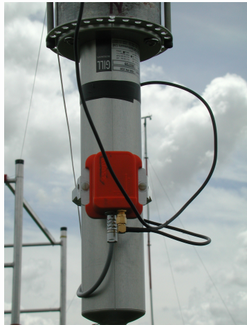
The turbulence tethersonde: sonic anemometer + inertial motion sensor (zoom ↓) + electronic system(house- made)
