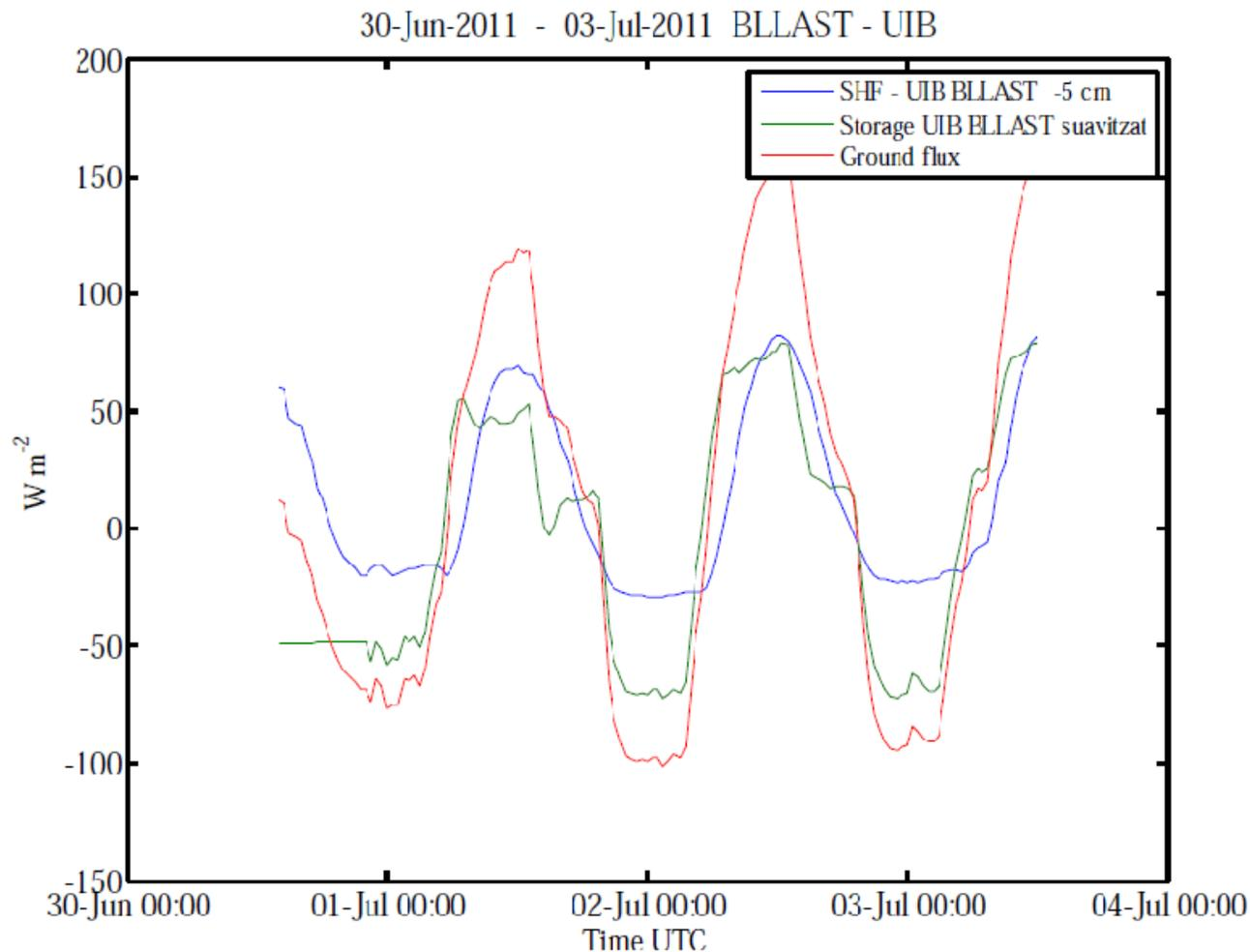
*Time evolution of the soil heat flux measured at 5 cm deep (blue), the storage term calculated from  $\Delta T$  with a moving average (green) and the resulting ground heat flux at the surface (red). Figure from Conangla, personal communication.*
