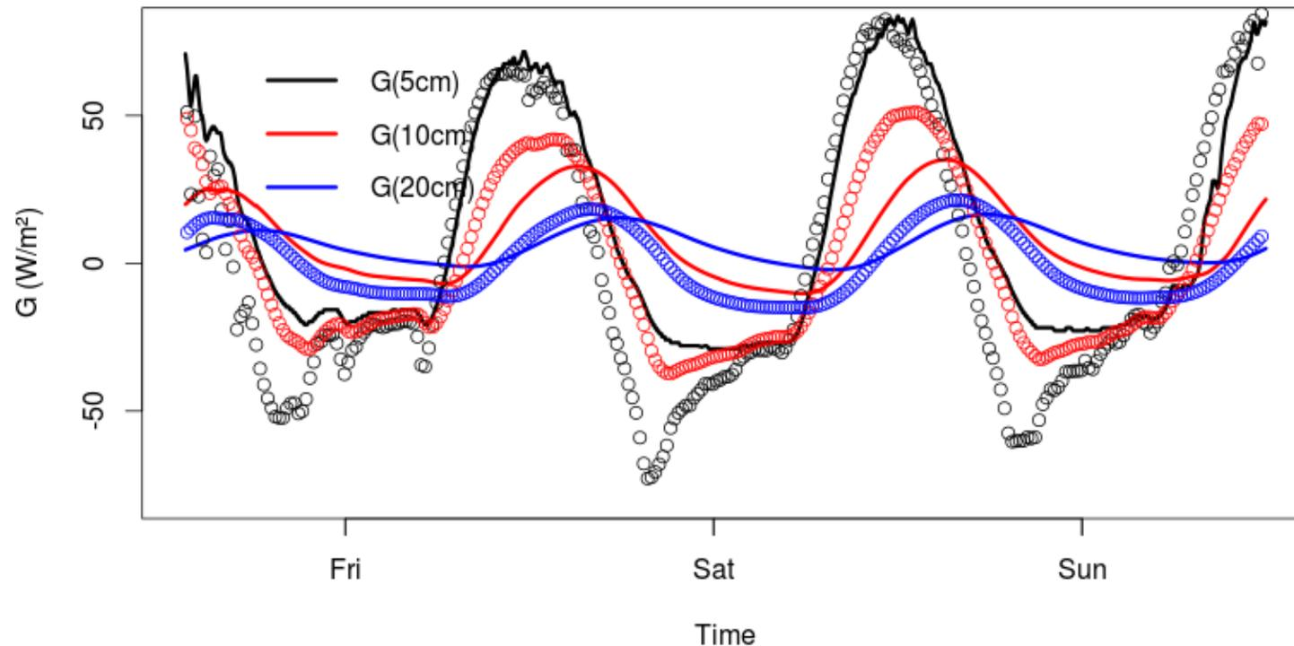
*Time evolution of the soil heat flux at 5 (black), 10 (red) and 20 (blue) cm deep estimated (dots) through the harmonic analysis with a fixed thermal diffusivity  $D_T = 5 \times 10^{-7} \text{ m}^2 \text{ s}^{-1}$  and a thermal conductivity  $\kappa = 0.4 \text{ W m}^{-1} \text{ K}^{-1}$ . Filled lines represent the corresponding measurements.*
