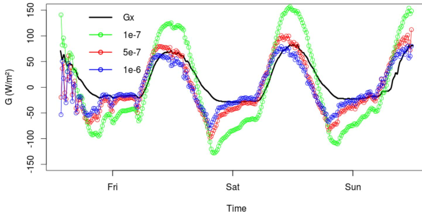
*Estimated soil heat flux at 5 cm deep with a fixed thermal conductivity  $\kappa = 0.4 \text{ W m}^{-1} \text{ K}^{-1}$  and for different values of thermal diffusivity  $D_T$ :  $1 \times 10^{-7}$  (green),  $5 \times 10^{-7}$  (red) and  $1 \times 10^{-6} \text{ m}^2 \text{ s}^{-1}$  (blue). In black, the experimental heat flux measured at 5 cm deep.*
