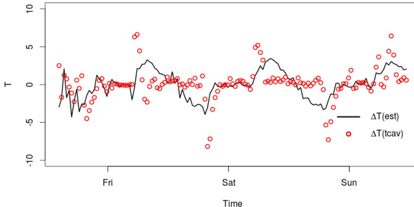
Time evolution of the difference of temperature  $\Delta T = T_f - T_i$  of the soil layer measured by TCAV (red) or estimated by the harmonic method (black) with a fixed thermal diffusivity  $D_T = 5 \times 10^{-7} \text{ m}^2 \text{ s}^{-1}$ .
