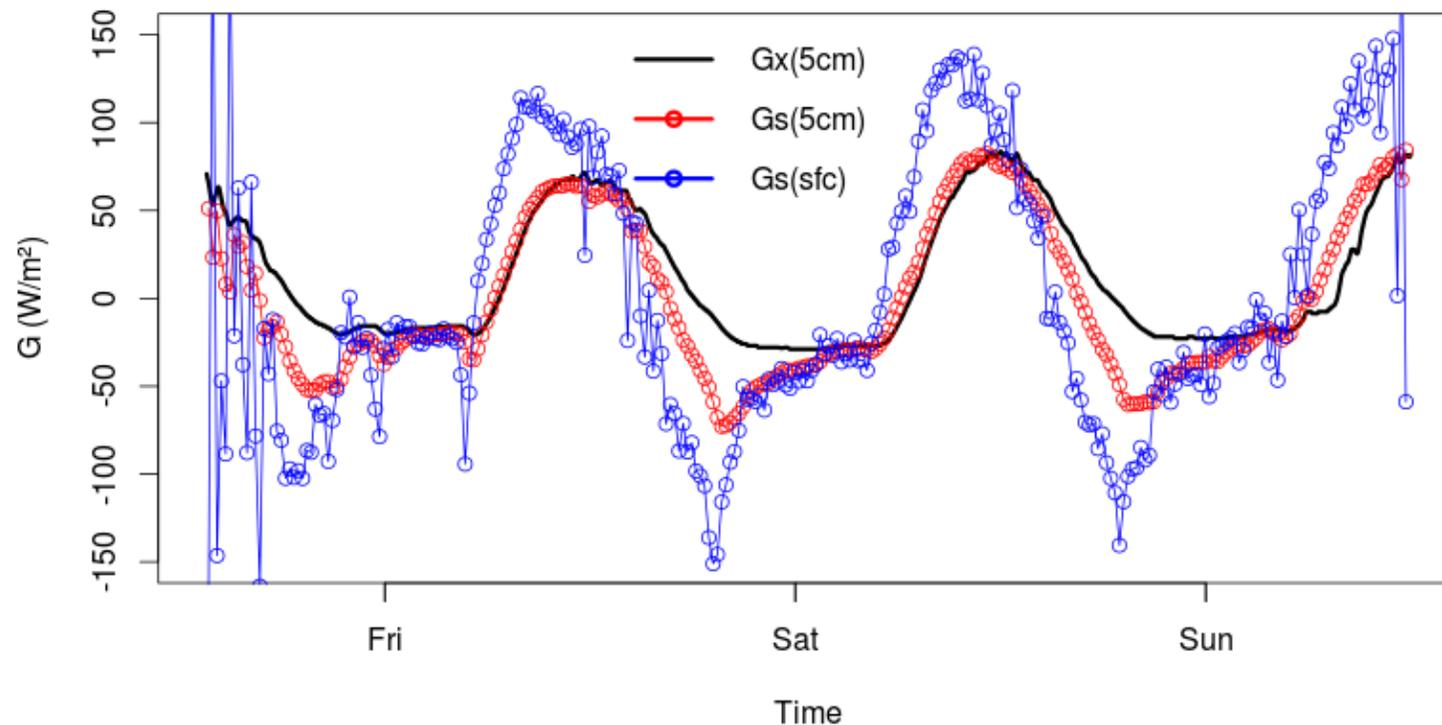
*Estimated soil heat flux at 5 cm deep (red) and at the surface (blue) with a fixed thermal diffusivity  $D_T: 5 \times 10^{-7} \text{ m}^2 \text{ s}^{-1}$  and thermal conductivity  $\kappa = 0.4 \text{ W m}^{-1} \text{ K}^{-1}$ .*
