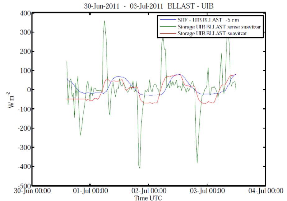
a) Time evolution of the bulk temperature  $T$  of the upper soil layer measured by TCAV (blue) and the corresponding temperature difference  $\Delta T$  in the interval time  $\Delta t = 1800$  s (green). b) The measured soil heat flux at 5 cm deep (blue), the storage term calculated with the raw time series of  $\Delta T$  (green) and after applying a moving average of a window size of 30 min to  $\Delta T$  (red). Figures from Conangla, personal communication.
