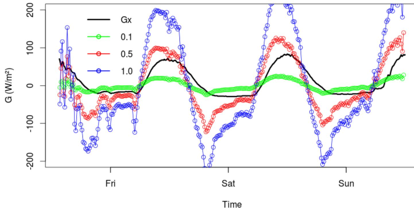
*Estimated soil heat flux at 5 cm deep with a fixed thermal diffusivity  $D_T: 5 \times 10^{-7} \text{ m}^2 \text{ s}^{-1}$  and different values of thermal conductivity  $\kappa$ : 0.1 (green), 0.5 (red) and 1.0  $\text{W m}^{-1} \text{ K}^{-1}$  (blue).*
