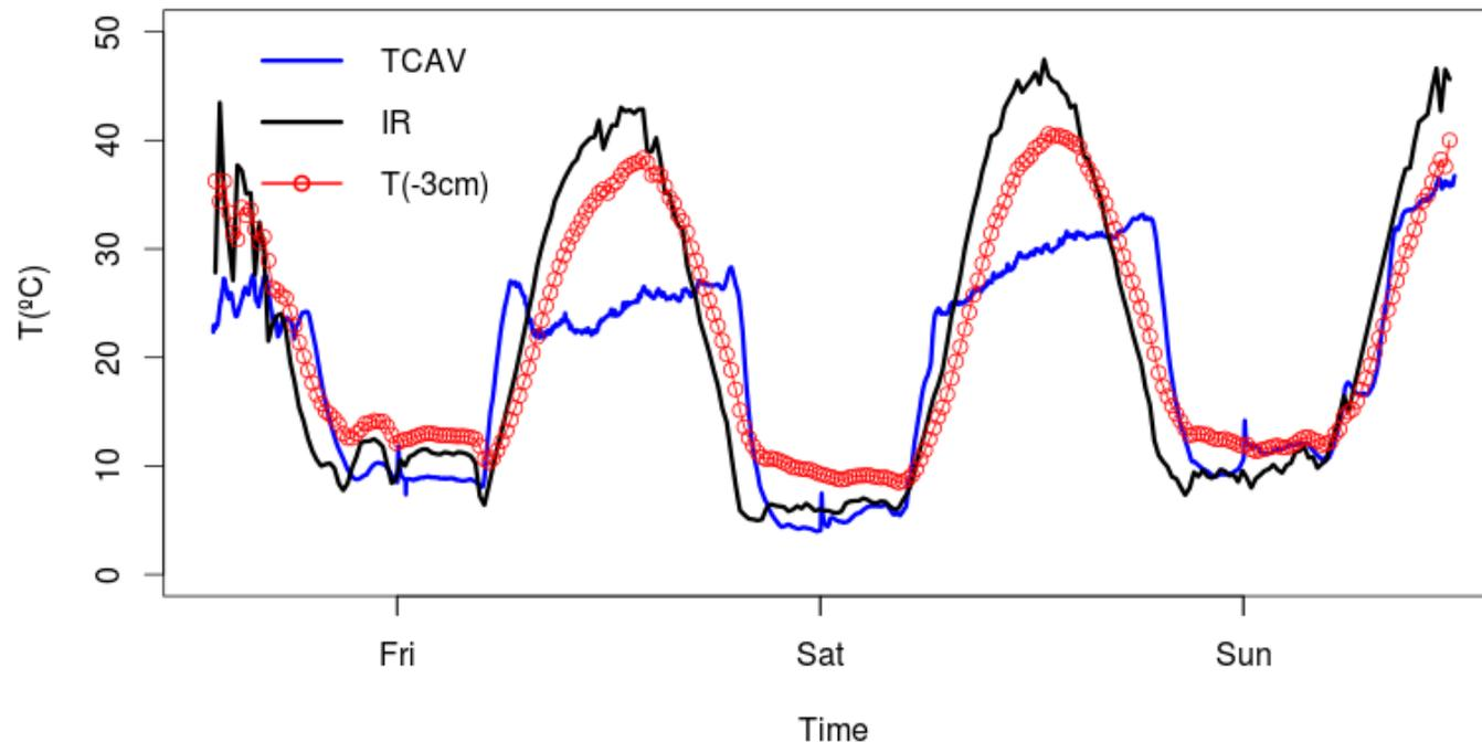
*Time evolution of surface temperature measured by the IR thermometer (black), temperature of the upper soil layer measured by TCAV (blue) and temperature of the soil at 3 cm deep estimated through harmonic analysis (blue) with a fixed thermal diffusivity  $D_T = 5 \times 10^{-7} \text{ m}^2 \text{ s}^{-1}$ .*
